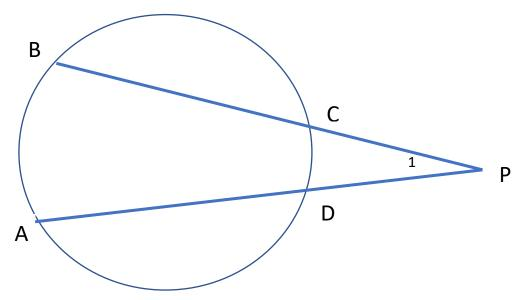
When two secants are drawn to a circle from an exterior point, the measure of the angle formed is equal to half the sum of the intercepted arcs
